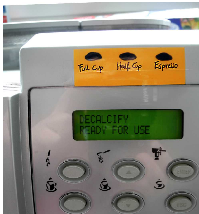
Figure 3.1: A coffee machine with added instructions on an orange note, telling that the buttons are for “Full Cup”, “Half Cup”, “Espresso”.
